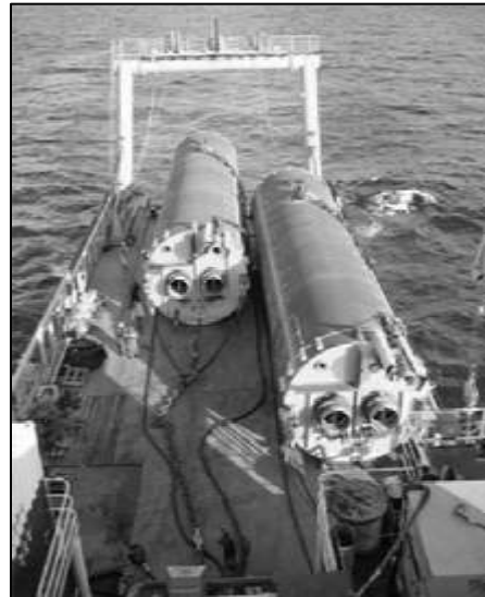
Suction anchors ready to be deployed.
