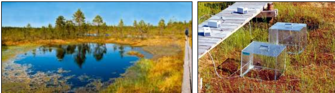
Flux chambers to sample gas emissions
