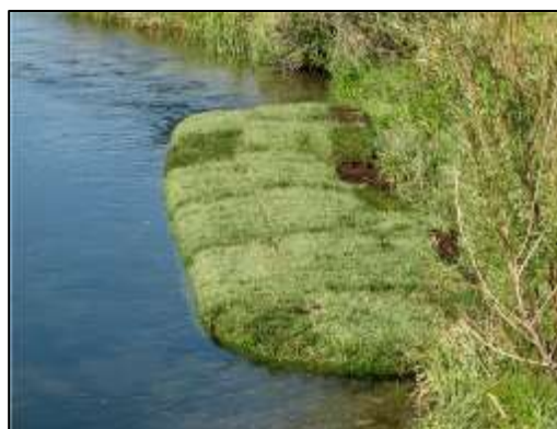
A smaller FTW under test as a means of bank stabilization.
