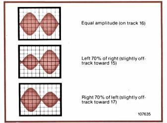
Figure 1. No Head Radial Alignment Necessary
