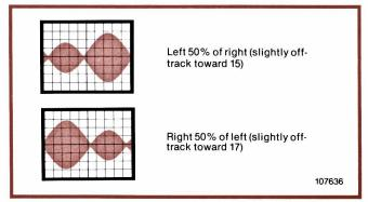
Figure 2. Head Radial Alignment Necessary
